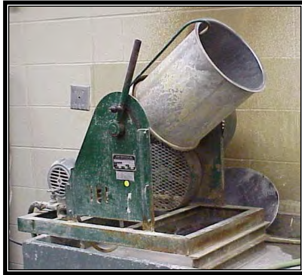
Figure 10-2. Mechanical Decant Device
