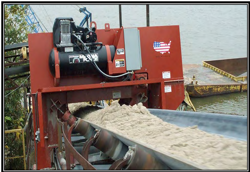
Figure 9-2. Belt Sampling with Mechanical Device
