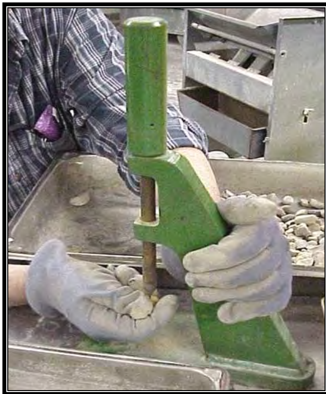
Figure 10-5. Scratch Hardness Tester
