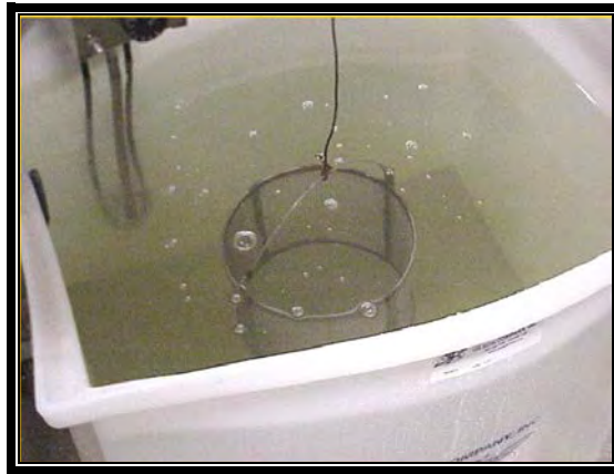
Figure 1 Coarse Aggregate Gravity Apparatus
