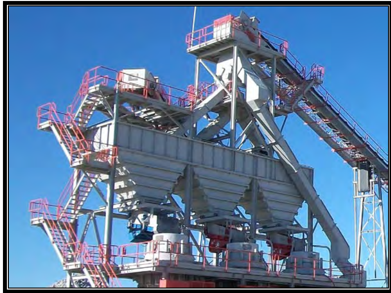
Figure 5-10. Crusher Feed System
