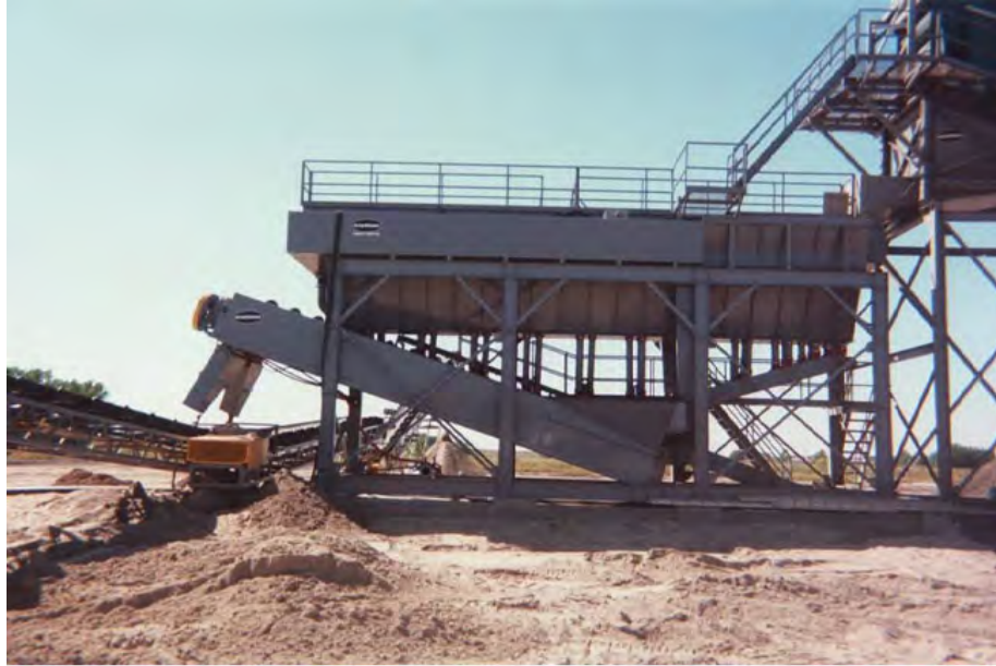
Figure 5-21. Multiple Cell Classifier
