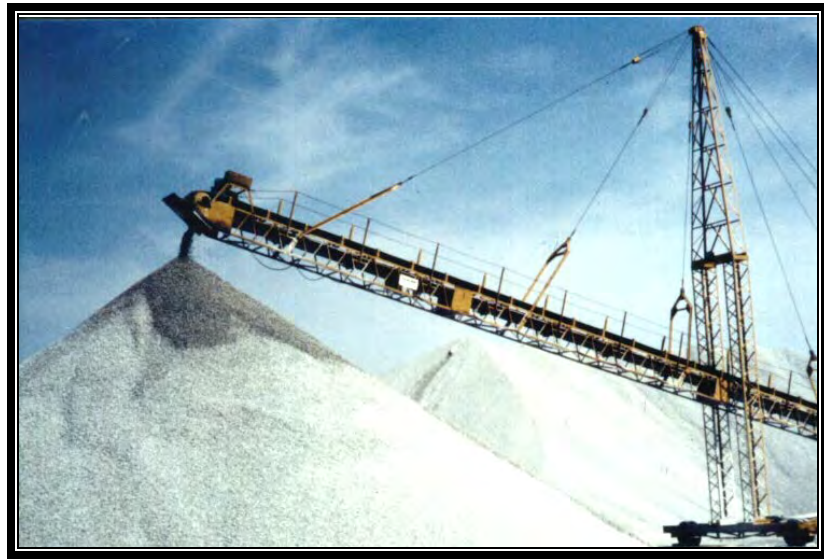
Figure 5-23. Adjustable Conveyor with Mixing Paddle
