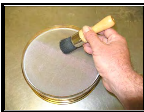
Figure 4 Use Hair Brush on Fine Sieves
