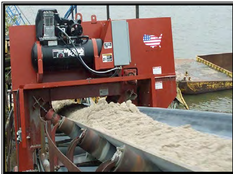
Figure 3 Automatic Sampling Device
