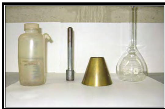
Figure 1 Fine Aggregate Specific Gravity Apparatus
