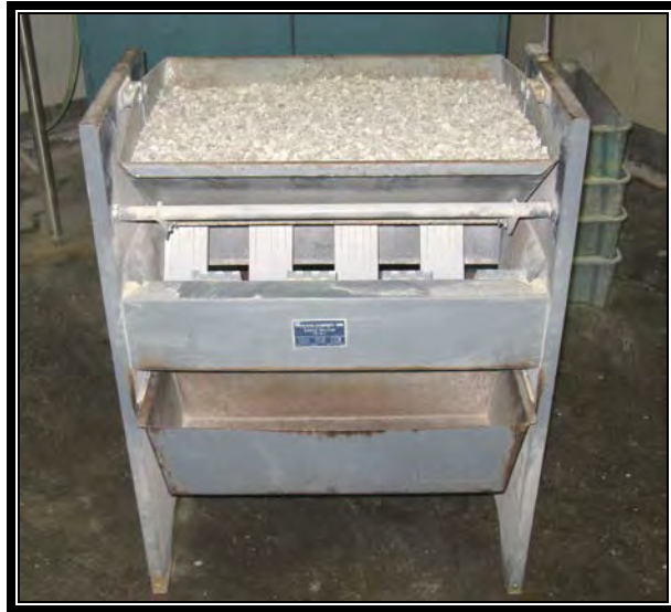
Figure 9-3. Mechanical Splitter
