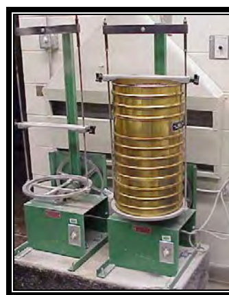
Figure 2 Small Sieve Shaker
