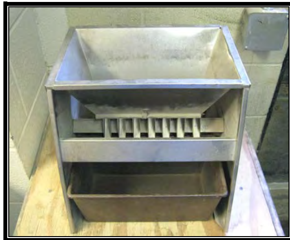
Figure 9-4. Sand Splitter
