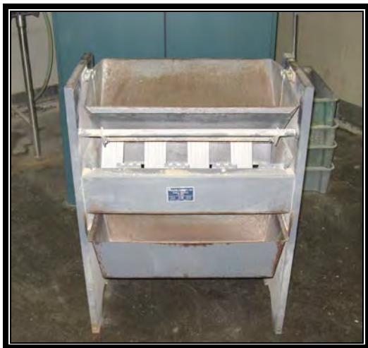
Mechanical Splitter
